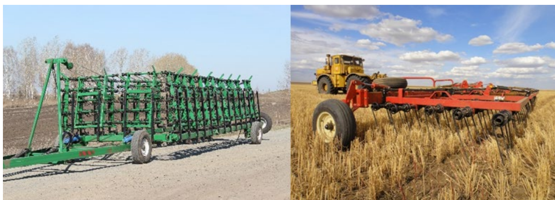
Figure 25: Heavy harrow for modern straw management. (Source: Own photos).
