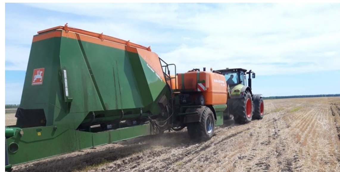
Figure 38: Cart for liquid fertilizer between tractor and seed drill. (Source: Own photo).
