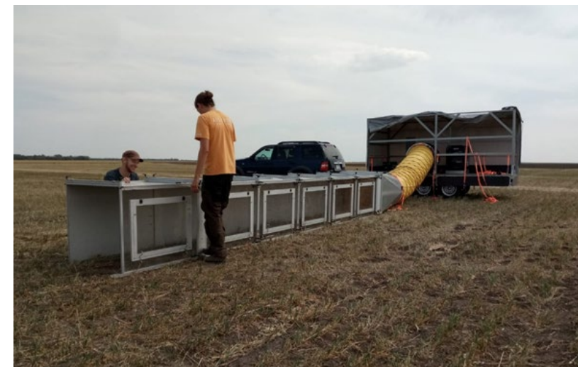
Figure 13: Mobile wind generator to measure wind erosion. (Source: G. Schmidt, 2019).
