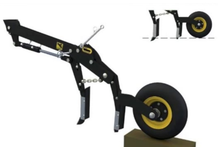
Figure 37: Coulter system with two openers. (Source: Väderstad, 2019, https://www.vaderstad.com/en/drilling/seed-hawk-air-seeders/seed-hawk-opener/ ).
