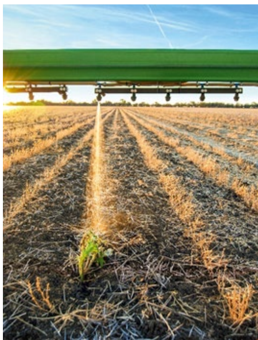
Figure 45: On-point weed treatment using the AmaSpot system. (Source: Own photo).
