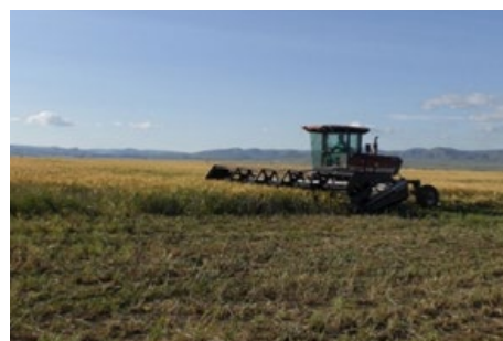
Self-propelled Macdon swather 100 hp wide row
