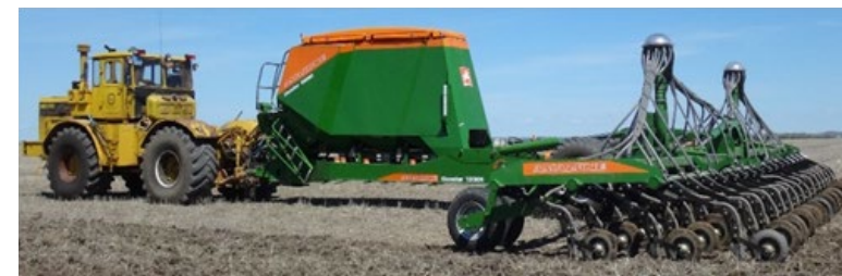
Figure 32: Condor 12001 seed drill for direct seeding by Amazonen-Werke with Russian tractor K700A. (Source: Amazonen -Werke, 2012).
