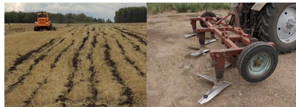
Figure 24: Flat-cutting wing blade cultivators do not break up the soil and cut the roots of the weeds and self-sown crops in Aleysky District, Altai Krai. (Source: Own photos).
